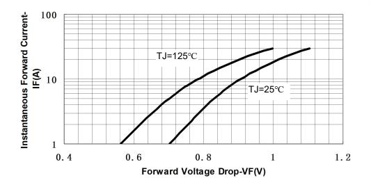
Fig.3-Typical Instantaneous Forward Voltage Characteristics
